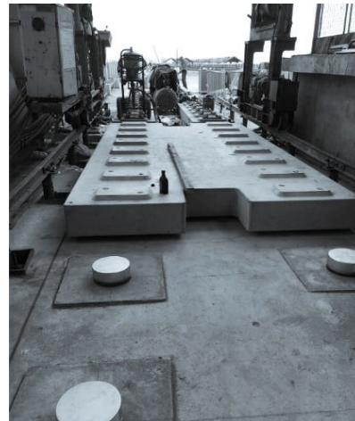
FST on Rubber Bearings: Ningbo Fengshua Line
